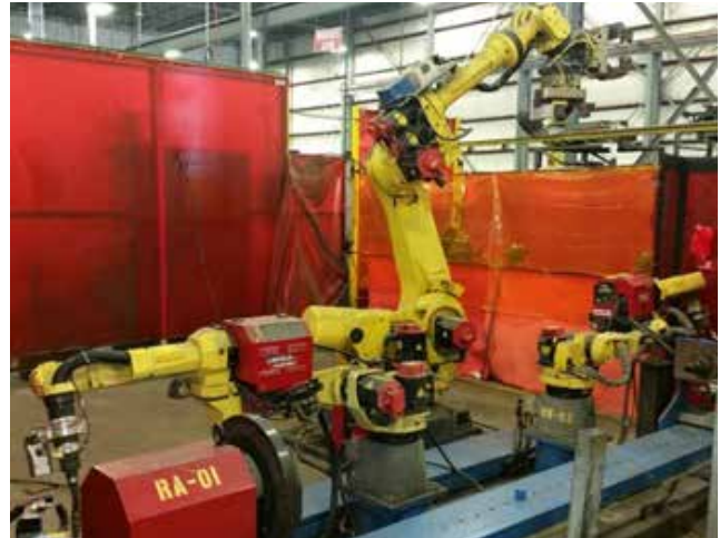
Robotic welding for consistent quality
